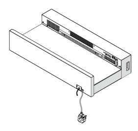
Insert the plug through the hole in the cover and reattach the cover.  $\label{eq:cover_plus}$
