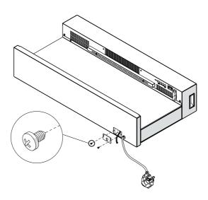
Place the fireplace on a flat surface and remove the two screws as shown. Open the cover on the base plate and remove the plug for mood light.
